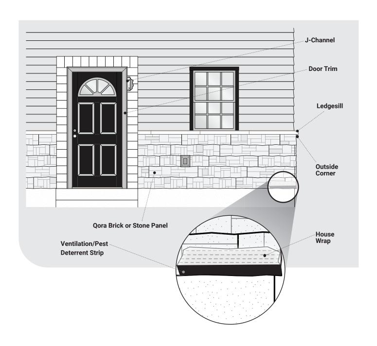
Before installing Qora Cladding, it is important to ensure the walls are flat, a weather-resistant barrier is installed, and openings are properly flashed. For attachment over walls where the air inside the structure is not conditioned, Qora Cladding can be installed directly over other cladding materials like DuraTemp®, T1-11 plywood, LP SmartSide® or steel siding where the weather barrier is integrated or unnecessary.
