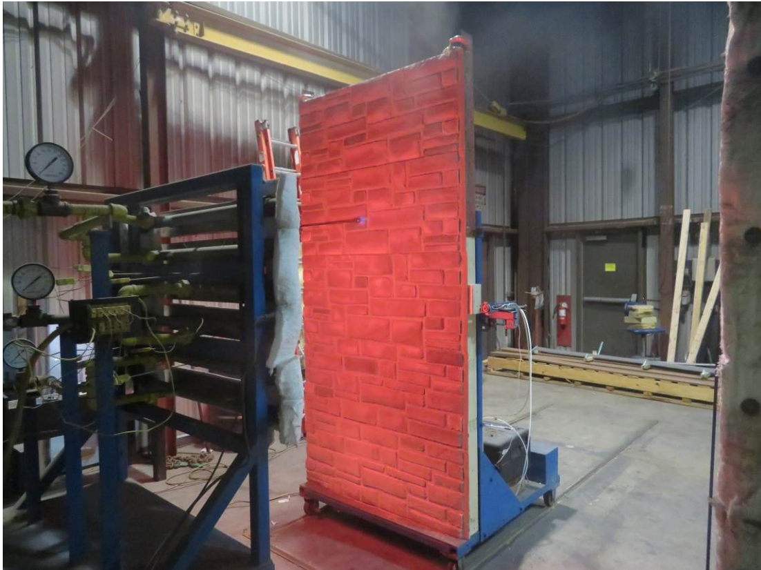
Figure B-2. Sample starting to smoke during fire exposure.
