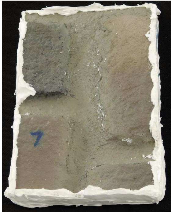
Sample #7 – At 336 hrs Humidity exposure IAW ASTM D2247-15 (see above)
